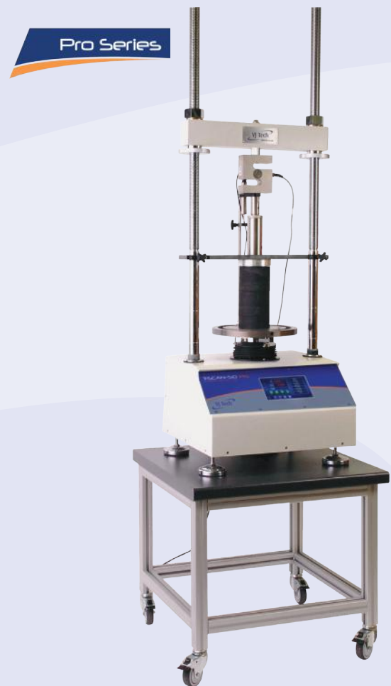
Unconfined Compressive Strength System Setup
