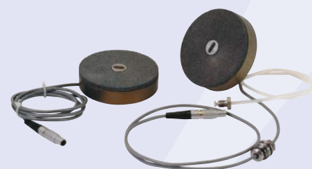
Bender Elements in 70 mm Top Cap and Base Pedestal
